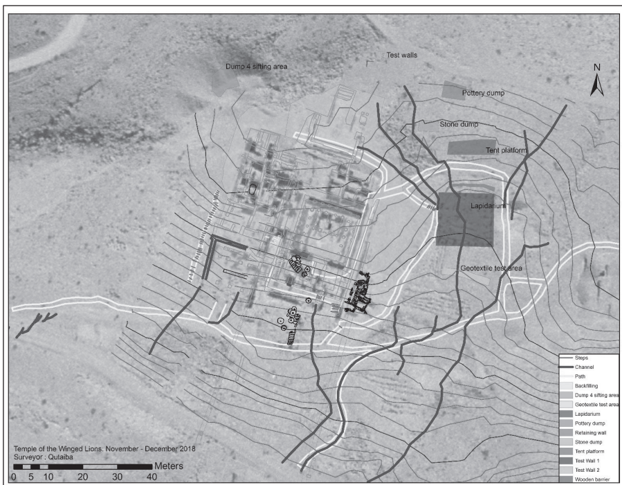
11. Composite contour map of the TWL, showing locations of features and interventions carried out as part of the TWLCRM Initiative, including paths, steps, backfilled areas (pink), and the presence of drainage channels (blue). Note the perpendicular drainage channels in the southwest quadrant (surveyed by Qutaiba Dasouqi, December 2018).
